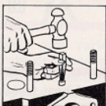
(2) Drive in P&C Extractor
